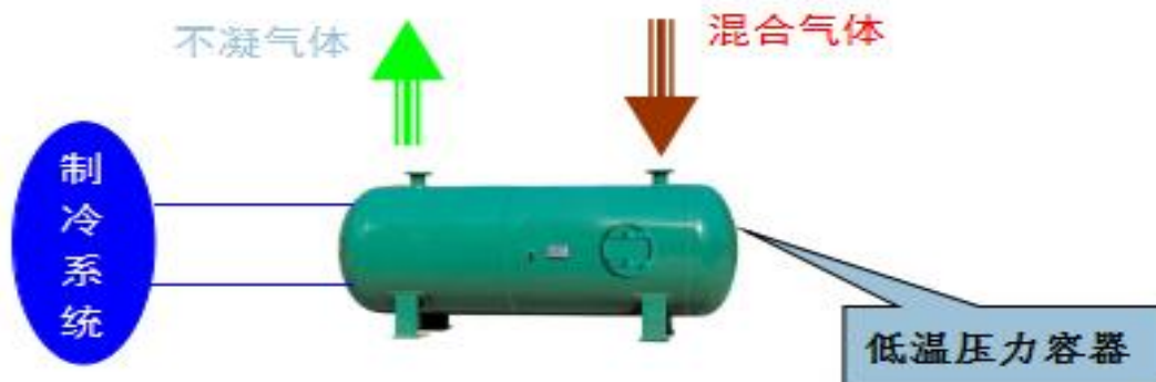
Figure 4-6 Low temperature distillation method schematic
