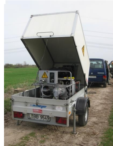
Electric power source TSQ4 ( I_{\max} = 11 \text{ A} , U_{\max} = 3.3 \text{ kV} )
