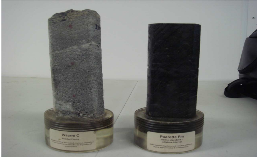
Photo 2: Core of Waarre C and Paaratte formation
