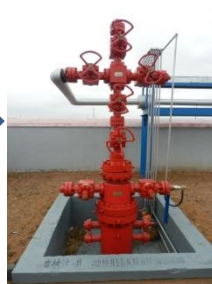
注入井 4个储层, 笼统注入 Injection well (4 reservoirs, general inject)
