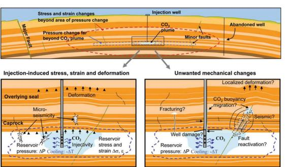
Any change in reservoir pore pressure will induce some stress and strain changes in and around the injection zone.
