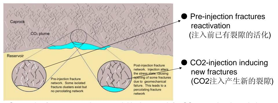
Connecting fractures supply a potential leakage path for CO2 escaping through the cap-rock. The mechanical integrity is considered to be damaged if the pre-fractures are activated or new fractures are induced.
