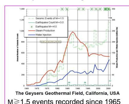
CO2 injection is similar with water injection, the geomechanical issues have received increasing attentions.
