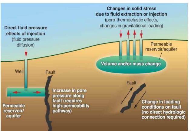
The effective stress acting on fault decrease by increasing pore pressure.
