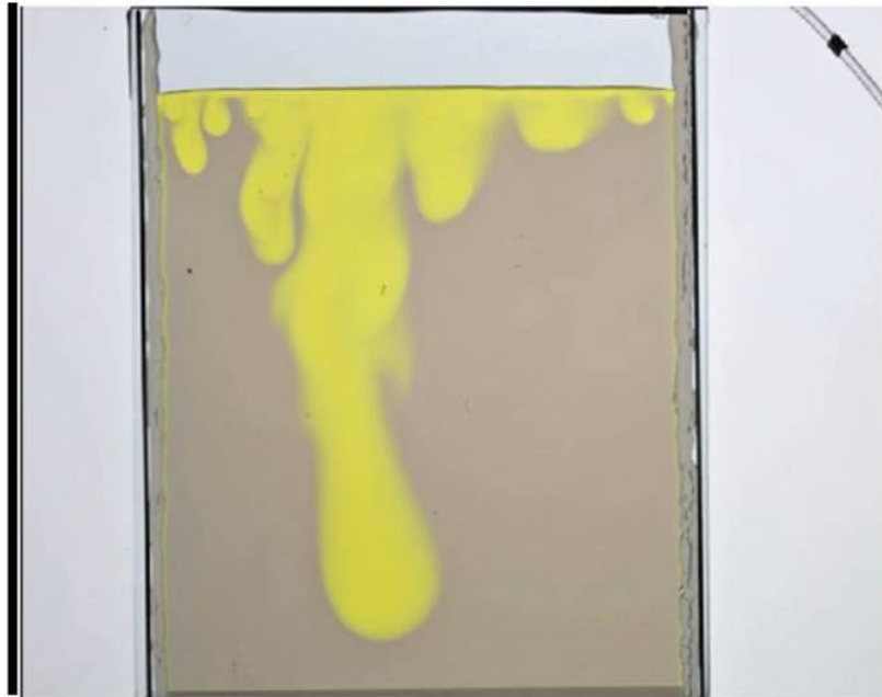
Lab test timelapse sequence showing plumes of denser CO 2 -rich water descending into CO 2 -poor water. Cell = 30x30 cm, test duration = 2 hours.
