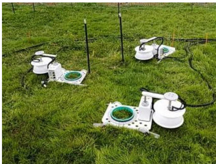
Monitoring CO 2 fluxes in experiments investigating impacts of CO 2 leaks on agricultural soils and crops
