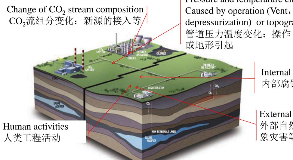
Pressure and temperature change in the pipeline : Caused by operation (Vent, shut-in and depressurization) or topography etc. 管道压力温度变化:操作(排放、关停、减压) 或地形引起
