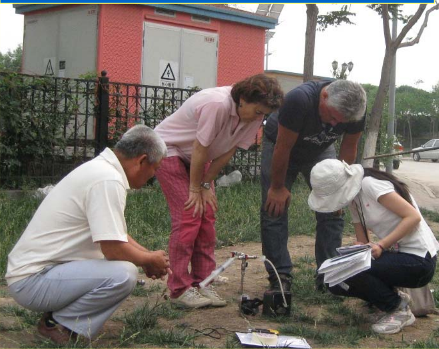
Soil gas sampling and measurement
