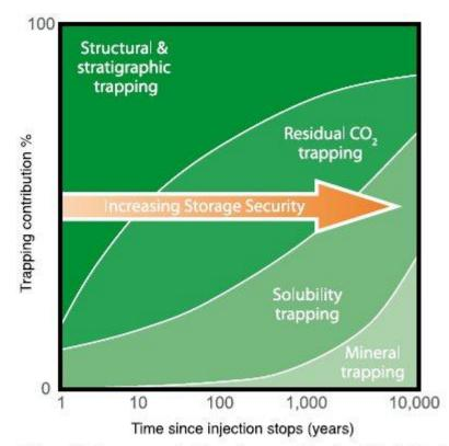
Figure 5.9 Storage security depends on a combination of physical and geochemical trapping. Over time, the physical process of residual CO, trapping and geochemical processes of solubility trapping and mineral trapping increase. **IPCC SRCCS 2005**
