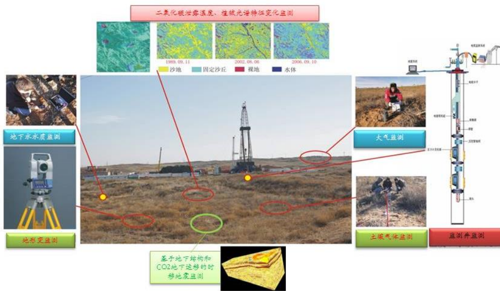
Fig.1 Monitoring system of CO2 storage
